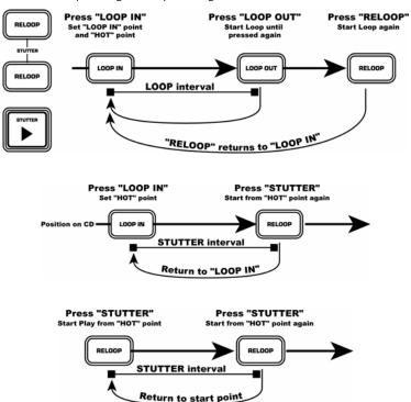
*NOTE: The CD Player will always remember a new set "Hot" points until you actually set a new "LOOP IN" point or put in a new CD. The new point will be accessible until you remove the <u>CD from the unit</u>. If you change*
